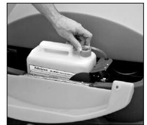
Attach the cap to bottle and detergent is automatically diluted to the proper ratio.
